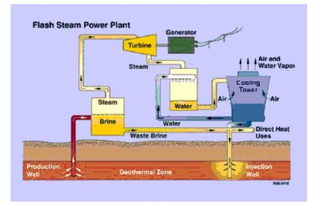
Figure 40: Diagram of Geothermal Power Plant with Water-Cooled System
