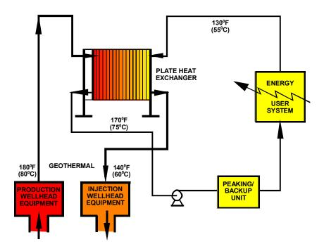
Figure 77: Typical Direct use Geothermal Heating System Configuration
