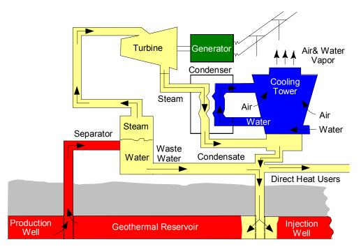
Figure 27: Single Flash Steam Power Plant Schematic
